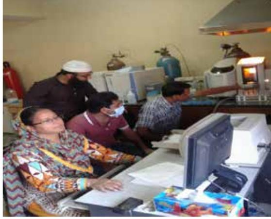
Atomic Absorption Spectrometer to detect heavy metals
