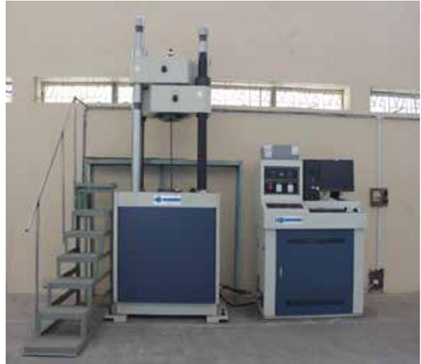
Universal Testing Machine (UTM) used for testing of MS rod, flat bar, concrete, block etc.
