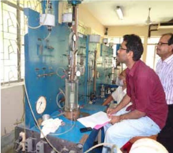
Triaxial Shear Test Apparatus used for determining Shearing strength of soil.
